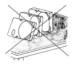
Do not place HDD vertically to avoid falling down.
